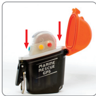
Unscrew two screws on top cap
